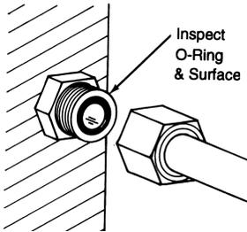
1. Inspect sealing surfaces and O-Ring groove for damage or foreign material. Check the O-Ring to insure that it is properly seated in the O-Ring groove.
