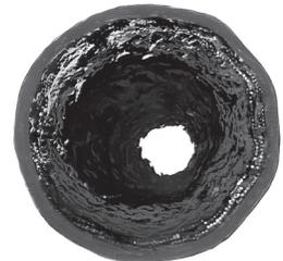
Indications are that the hose tube is not compatible with the agent being carried. Even though the agent is normally compatible, the addition of heat can be the catalyst that can cause inner liner deterioration. Consult your hose supplier for a compatibility list or present him with a sample of the fluid being conducted by the hose for analysis. Make sure that the operating temperatures both internal and external do not exceed recommendations.
