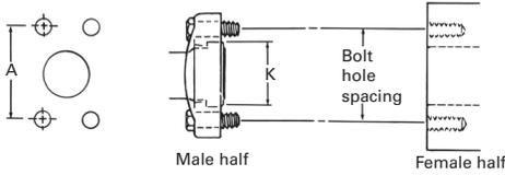
This connection is commonly used in fluid power systems. There are two pressure ratings. Code 61 is referred to as the "standard" series and Code 62 is the "6000 psi" series. The design concept for both series is the same, but the bolt hole spacing and flanged head diameters are larger for the higher pressure, Code 62 connection. The female (port) is an unthreaded hole with four bolt holes in a rectangular pattern around the port. The male consists of a flanged head,
