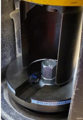
The T-400-MK conversion kit is designed to allow the use of standard Danfoss tooling, hose, and hose ends in the Parker Minikrimp crimper. Everything is included to convert the crimper to accept Danfoss tooling. This kit gives the crimper capacity to crimp up to and including 5/8" I.D. 2 wire braided and 5/8" I.D. 4 wire spiral factory-type hose assemblies.
