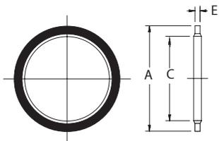
BSPP bonded seal for DIN 3852-2 ports
