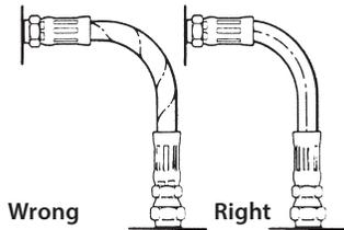
Minimum bend radius is measured on the inside bend of the hose. To determine minimum bend, divide the total distance between ends (B length) by 2. For example, B=6, minimum bend radius=3.
