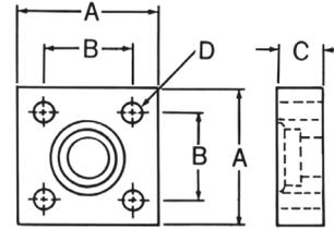
The JIS 4-bolt square flange connection is similar in concept to the SAE 4-bolt flange connection, except that the JIS bolt pattern is
