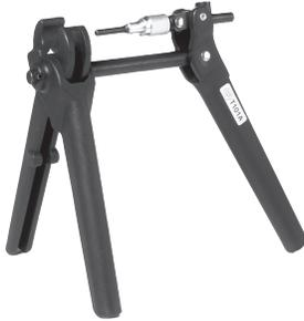
Assembly of Barb-Tite push-on hose ends is made easy with this handy tool. Easy and fast operation assures dependable, leak proof assemblies. Simply clamp hose in jaws, place hose end on push rod and pull the handle. Engineered for a lifetime of rugged service.
