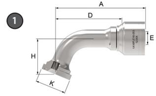
**Split Flange 67° tube elbow (SAE Code 61)**
