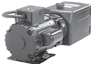
The T-441 power unit features a two-stage pump providing high flow at low pressure for a fast ram approach and low flow at high pressure for actual crimping.
