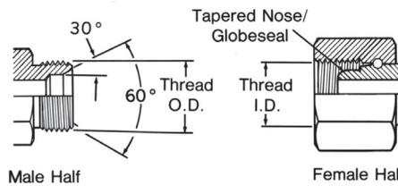
The BSP (parallel) male is similar to the NPSM male except the thread pitches are different in most sizes.
