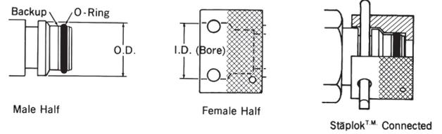
This is a radial O-Ring seal connection developed in Germany and commonly used for hydraulic application in underground mines. The male contains an exterior O-Ring and backup ring, plus a groove to accept the "staple". The female has a smooth bore
