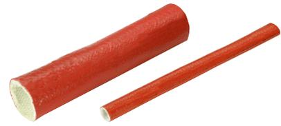
Firesleeve is a flame-resistant sheathing constructed of tightly woven fiberglass, which is coated with a specially compounded, highly temperature-resistant silicone rubber. Firesleeve offers protection in high temperature environments with heat extremes. It is not compatible with hydrocarbons.
