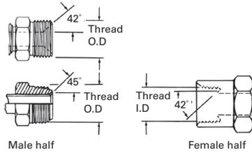
This connection is frequently used in automotive systems. The male connector can either be a 45° flare in the tube fitting form or a 42° seat in the machined adapter form.
