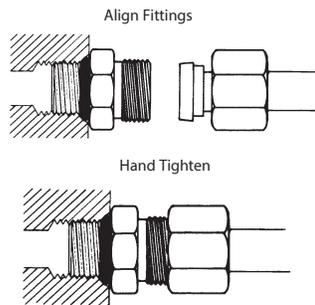
4. Complete the assembly by wrench tightening the nut to the recommended torque value on page 372.
