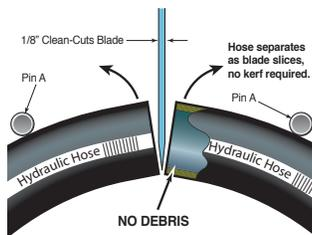
ET9100/200/300 hydraulic hose cutting system is break-through technology using a toothed blade, cutting with the backs of each tooth, so the blade does not take a kerf. The saw bends the hose into the blade spreading the cut edges to avoid burning and smoking.
