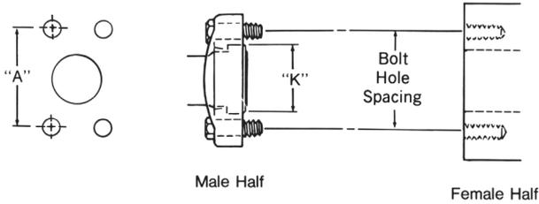
This connection is commonly used in fluid power systems. There are two pressure ratings. Type I (Code 61) is referred to as the "standard" series and Type II (Code 62) is the "6000 psi" series. The design concept for both series is the same, but the bolt hole spacing and flanged head diameters are larger for the higher pressure, Type II connection. Both metric and inch bolts are used. The female (port) is an unthreaded hole with four bolt holes in a rectangular
