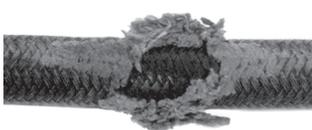
The primary function of the cover is to protect the reinforcement. Elements that may destroy or remove the hose covers are:
