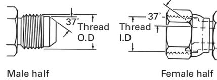
This connection is very common in fluid power systems. Both the male and female halves of the connections have 37° seats. The seal takes place by establishing a line contact between the male flare and the female cone seat. The threads
