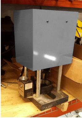
The T-420-GT conversion kit is designed to allow the use of standard Danfoss tooling, hose, and hose ends in the Gates PC707 crimper. Everything is included to convert the crimper to accept Danfoss tooling. This kit gives the crimper capacity to crimp up to and including 1-1/4" I.D. 4 wire spiral hose factory-type hose assemblies.
