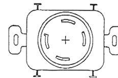
To obtain corresponding female wall receptacle order T-421-FP. For use with T-421U, T-441 and T-433 pumps.
