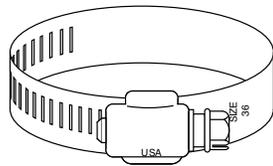
Partial stainless steel clamps utilize a 300 Series stainless steel band and housing with a steel case-hardened, zinc-plated screw. They feature a 14.3mm (9/16") band housing with a 8mm (5/16") hexagon and screwdriver slotted screw.
