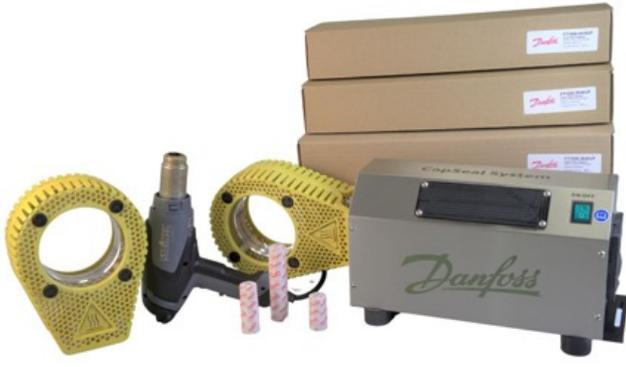
The FT1555 CapSeal system is intended to be used in conjunction with the FT1355 and FT1455 series projectile cleaning systems to prevent recontamination of hose, tube, and pipe assemblies. The FT1555 CapSeal system utilizes heat shrink technology to encapsulate the end of a hose or tube assembly with an FT1555 CapSeal capsule.
