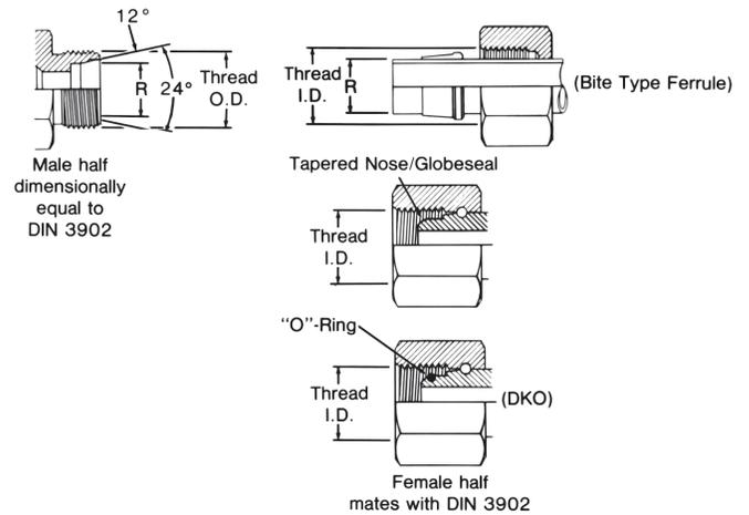
This connection style consists of a common male and three different female halves. The male has a straight metric thread, a 24° included angle and a recessed counterbore that matches the tube O.D. used with it. The female may be a tube, nut and
