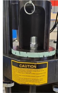
The T-420-KK conversion kit is designed to allow the use of standard Danfoss tooling, hose, and hose ends in the Parker Karrykrimp 1 and Karrykrimp 2 crimpers. Everything is included to convert the crimper to accept Danfoss tooling. This kit gives the crimper capacity to crimp up to and including 1" I.D. braided hose and 5/8" I.D. 4 wire spiral hose for the Karrykrimp 1 and up to and including 1 1/4" I.D. 4 wire spiral hose for the Karrykrimp 2.
