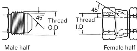
This connection is commonly used in refrigeration, automotive and truck piping systems. The connector is frequently made of brass. Both the male and female connectors have 45° seats. The seal takes place between the male flare the female
