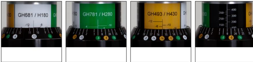
This machine is designed to easily adjust to Danfoss' core products. It's as simple as turning the collar to the correct color to match the layline on the hose, adjust the ring so that the correct size dot aligns with the correct size line on the collar and the machine is set for the correct crimp. Load the correct crimp die based on the crimp die chart attached to the machine, and the machine is ready to crimp.
