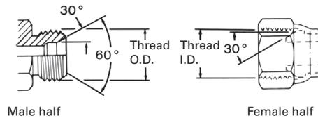
This connection is still widely used in fluid power systems, even though it is not recommended by the National Fluid Power Association (NFPA) for use in hydraulic applications. The thread
