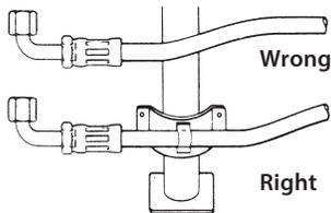
Install hose runs to avoid rubbing or abrasion. Use Weatherhead Hose Clamps to support long runs of hose or to keep hose away from moving parts. It is important that the clamps not allow the hose to move. This movement will cause abrasion and premature hose failure. (See Hose Clamps page 241 - 243)
