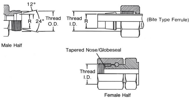
This connection consists of a common male and two different females. The millimetric series is used with whole number
