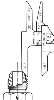
Measure the thread diameter with an I.D./O.D. caliper as shown. Match the measurements to the charts.
