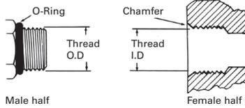
This port connection is recommended by the NFPA for optimum leakage control in medium and high pressure hydraulic systems. The male connector has a straight thread and an O-Ring. The female port has a straight thread, a machined
