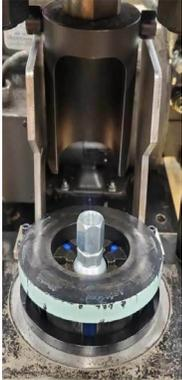
The T-420-PK conversion kit is designed to allow the use of standard Danfoss tooling, hose, and hose ends in the Parker Parkrimp 1 crimper. Everything is included to convert the crimper to accept Danfoss tooling. This kit gives the crimper capacity to crimp up to and including 1" I.D. braided hose and 5/8" I.D. 4 wire spiral hose.
