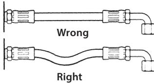
Keep the bend radius of the hose as large as possible to avoid collapsing of the hose and restriction of flow. Follow catalog specs on minimum bend radii.
