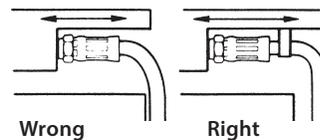
Use elbows and adapters in the installation to relieve strain on the assembly and to provide easier and neater installations that are accessible for inspection and maintenance.
