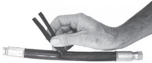
This would indicate that the pressure has exceeded the minimum burst strength of the hose. Either a stronger hose is needed or the hydraulic circuit has a malfunction which is causing unusually high pressure conditions.
