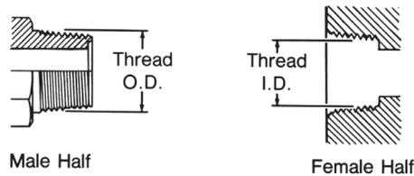
This BSPT (tapered) connection is similar to the NPT, except that the thread pitches are different in most sizes, and the thread form and O.D.s are close but not the
