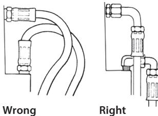
Make sure relative motion of the machine components produces bending rather than twisting of the hose. Hose should be routed so that the flex is in the same plane as the equipment movement.
