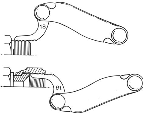
**Female** connections are usually measured by inserting the gauge into the connection and placing it on the sealing surface. If the centerlines of the connection and gauge are parallel, the correct angle has been determined.
