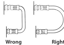
Do not twist hose during installation. This can be determined by the printed layline on the hose. Pressure applied to a twisted hose can cause hose failure or loosening of connections.
