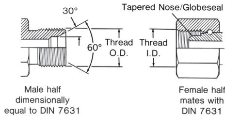
This connection is frequently used in hydraulic systems. The male has a straight metric thread and a 60° (included angle) recessed cone. The female has a straight thread and a tapered Nose/Globeseal seat. The seal takes place by contact between the cone
