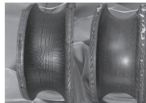
Heat has a tendency to leach the plasticizers out of the tube. This is a material that gives the hose its flexibility or plasticity.
