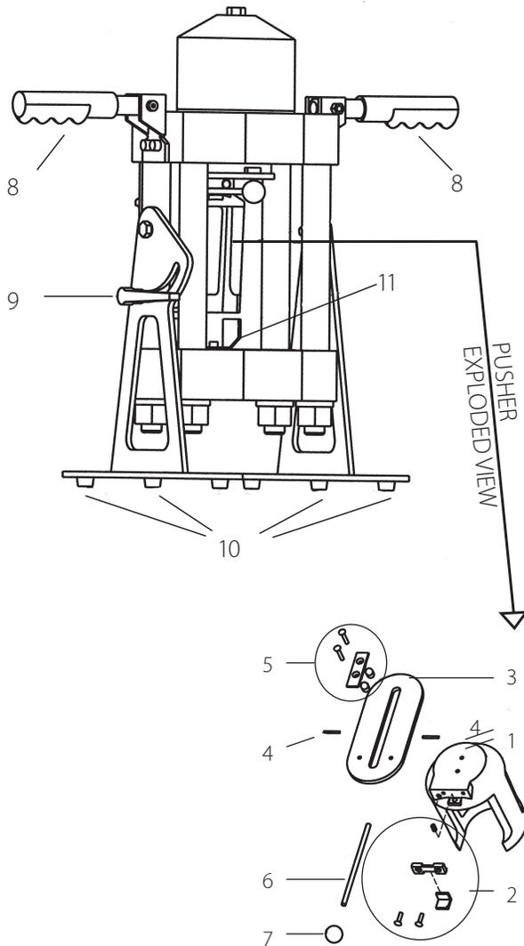
**T-480 portable crimp machine repair & replacement items**
