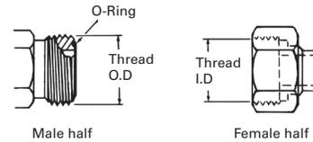
This connection offers the very best leakage control available today. The male connector has a straight thread and an O-Ring in the face. The female has a straight thread and a machined flat face.
