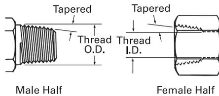
The JIS tapered thread is similar to the BSPT connection in design, appearance and dimensions. The JIS tapered thread and the BSPT connection are interchangeable.
